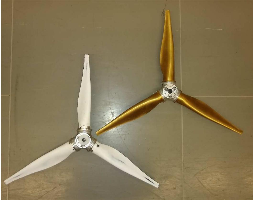
*Figure 23: CANOE carbon fibre and SSPA bronze blade, original geometry*
