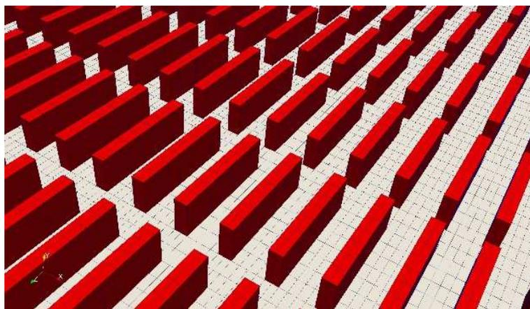
Figure 89 Surface mesh over the raised textures.
