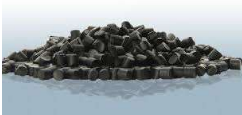
Commercial pellets (25wt% of CNT inside matrix)
