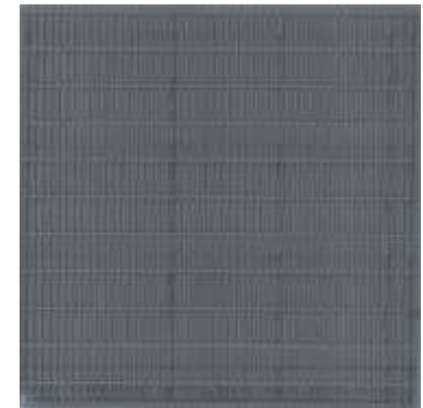
Figure 3. 3-D printed micro-texture taken using Keyence 3D light microscopy
