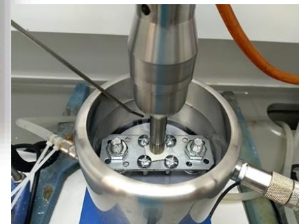
FUNDITEC's Set-up of cavitation erosion test
