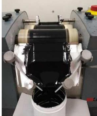
Figure 2. Dilution of CNT-masterbatch in NEMMO resin using 3 rolls mill.
