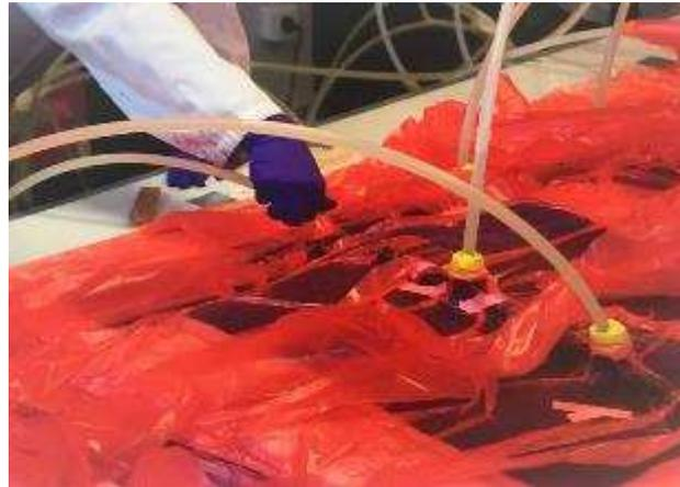
Figure 8. Picture of infusion process.
