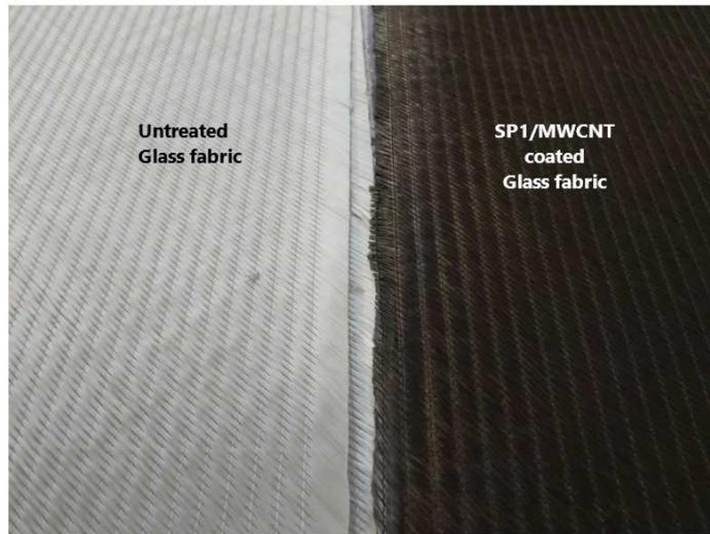
Figure 5. Visual inspection of the coating: homogeneous.
