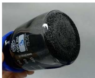
Figure 36. Problems observed during dispersion tests: sedimentation and non-dispersed particles.
