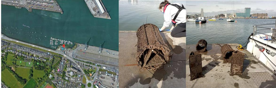
Figure 18. Left: Satellite imagery of the deployment location at Poolbeg Yacht & Boat Club, Dublin. Right: Images of triangular deployment cage used for housing glass slides (to avoid location effects).
