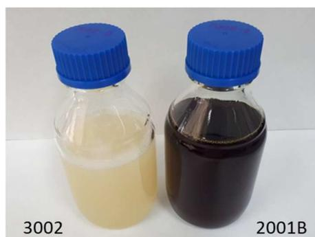
Figure 31. Acrylated (3002) and fluorinated (2001B) polyisocyanates synthesised by FUNDITEC.
