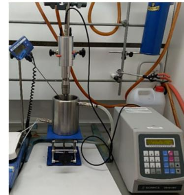
*FUNDITEC's Set-up of cavitation
