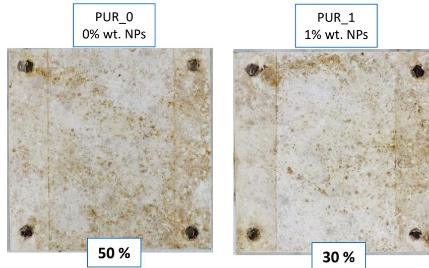
*The percentage cover of fouling was **reduced 20 %** compared to control system without nanoparticles*
