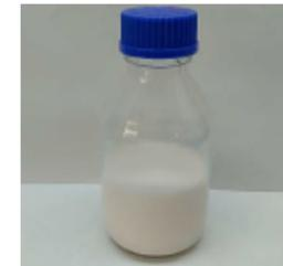
*Water-based polyurethane dispersion PUD5 synthesised by FUNDITEC*
