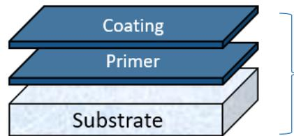
1x 100µm PU coating
