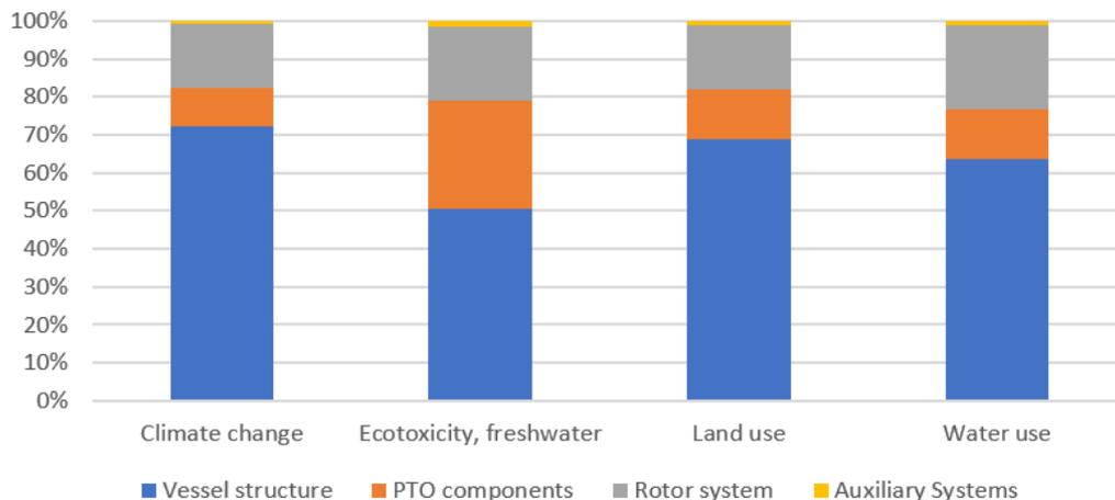
>50% of all categories of env. impacts are generated by the vessel structure (→ 360 tonnes of steel)
