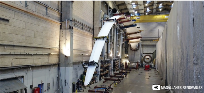
Figure 6: Blade breakage test.
