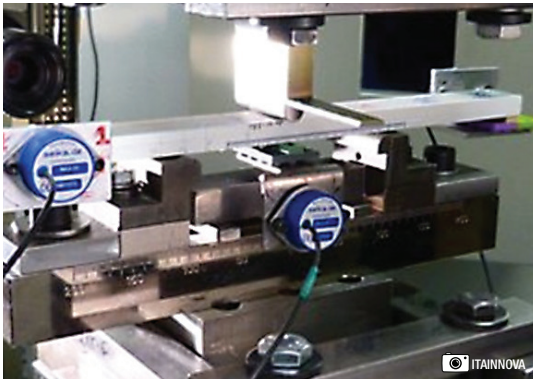
Figure 4: (left) Static test bench installed at ITAINNOVA. (right) Additive infusion process to fibreglass laminates.
