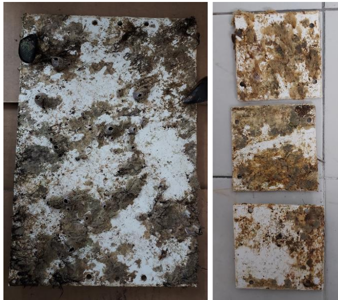
Figure 24: HarshLab Samples after 10 months of immersion before fouling cleaning
