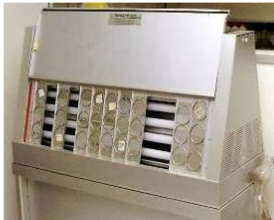
Figure 5: Tecnia chamber for UV/condensation ageing
