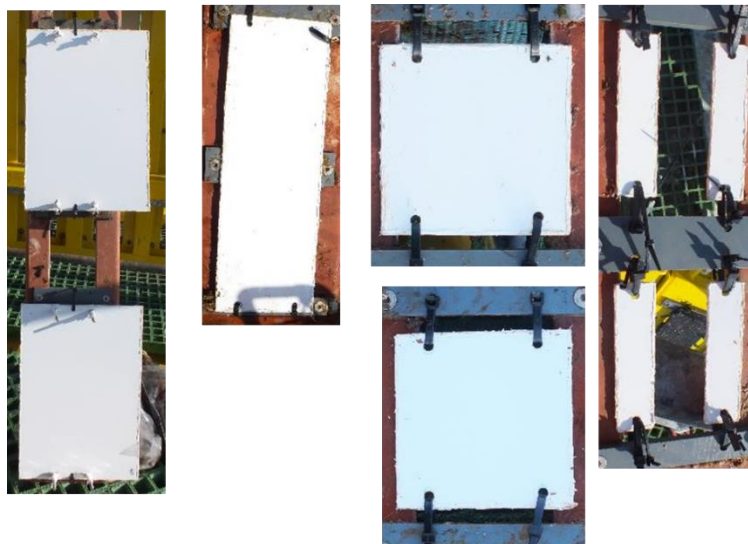
Figure 21: samples fixed on the rack before immersion, HarshLab, February 2020
