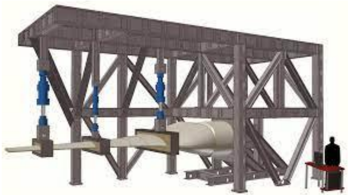
Figure 58: Traditional testing of tidal blades
