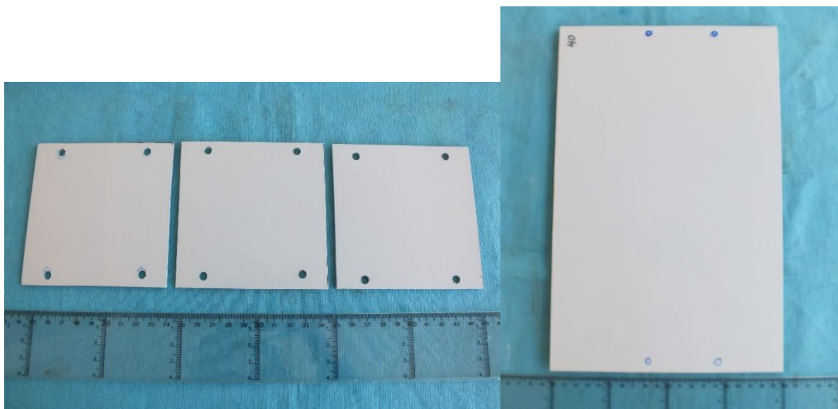
Figure 19: example of the aspect of the sample after machining: on the left: gravimetric sample for the HarshLab, on the right: panel to extract sample for tensile test after aging
