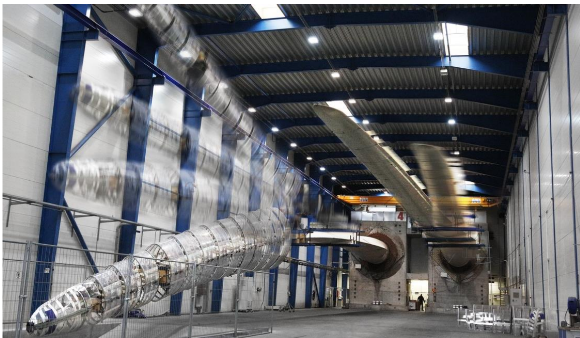
Figure 57: Fatigue testing of wind turbine blades (Source: LM Wind Power)
