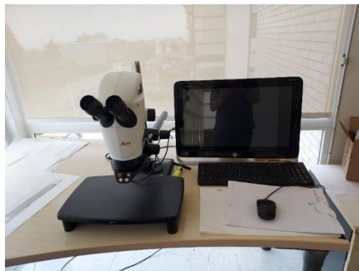
Figure 18: binocular setup with image acquisition system
