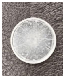
Figure 12: 1.2mm diameter KBr pellets with gelcoat powder for FTIR characterization
