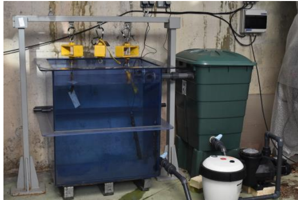
Figure 6: Tecnalia immersion tank for artificial ageing
