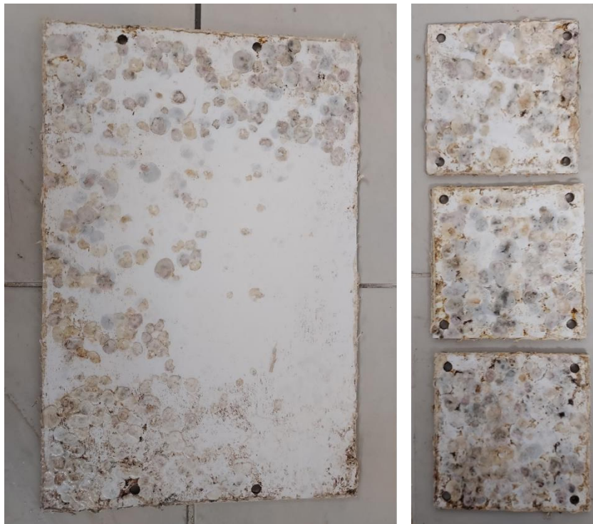
Figure 31: Aspect of the samples immersed in the port of Pasaia after cleaning
