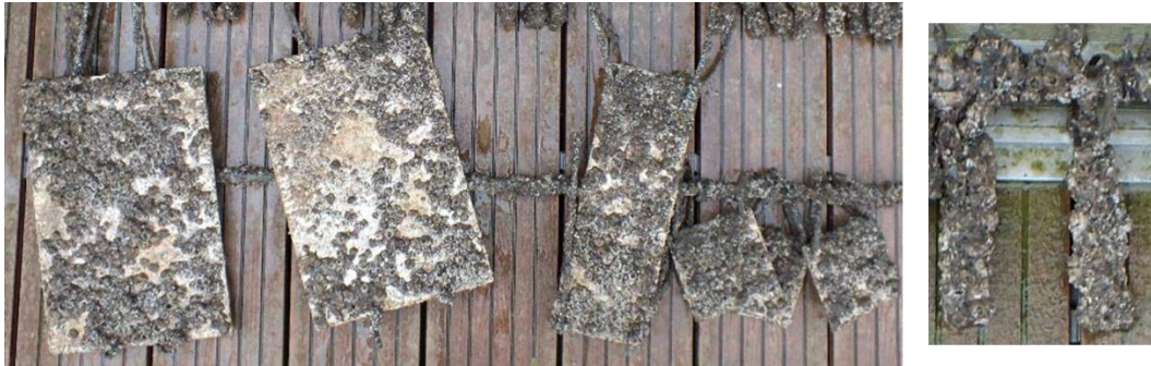
Figure 28: aspect of the samples immersed on the Pasaia port facility after 8 months of ageing
