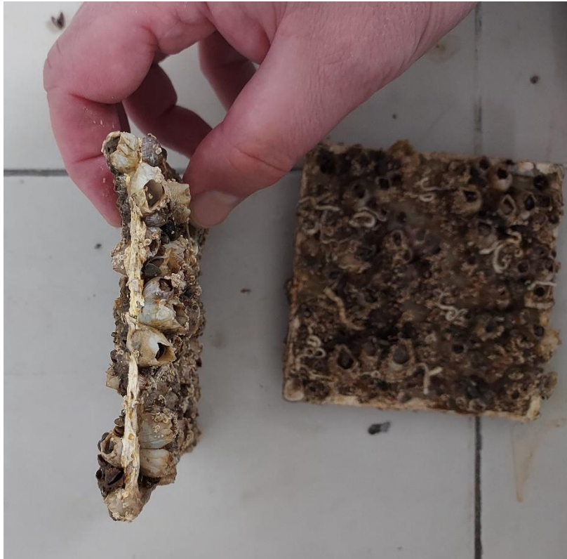
Figure 30: section of a sample exposed in the port of Pasaia for 10 months.
