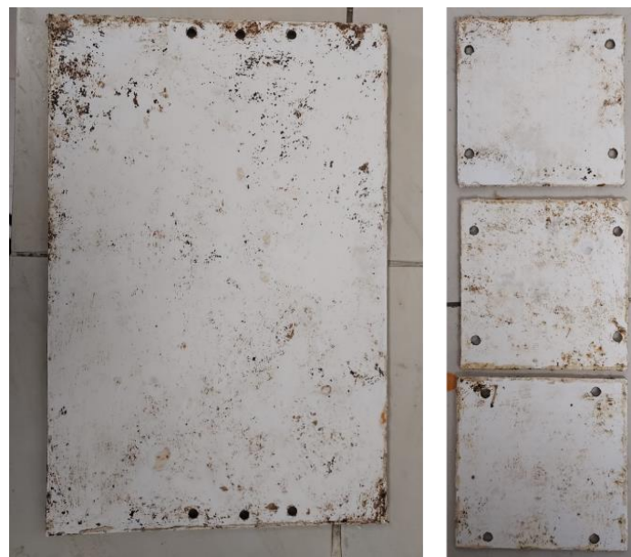
Figure 25: HarshLab Samples after 10 months of immersion after fouling cleaning
