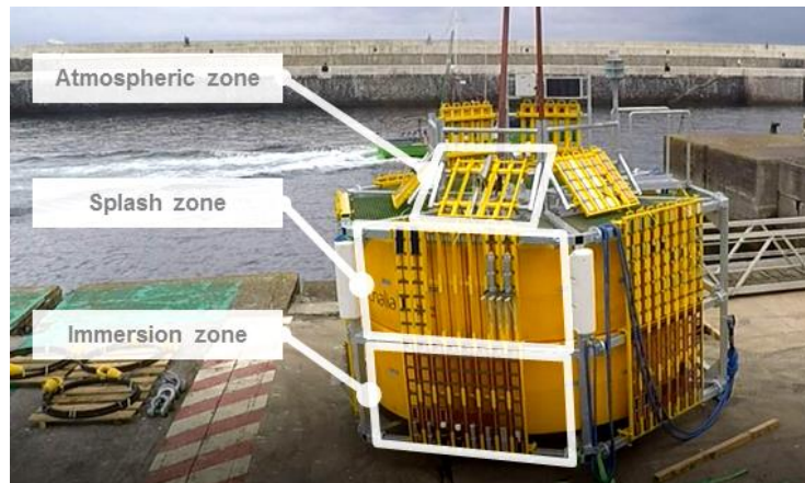
Figure 2: aspect of the HarshLab before installation, view on the immersion area
