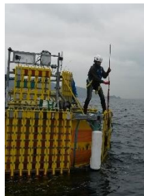
Figure 3: manipulation of the immersed racks to access to the immersed samples
