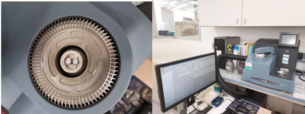
Figure 11: on the left: samples container in the sample holder of the DSC device (one is the reference and the other contains the gelcoat sample), on the right an overview of the DSC device used
