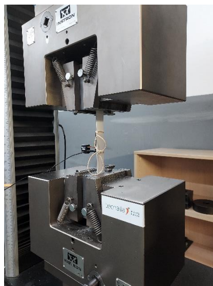
Figure 40: sample during the tensile test
