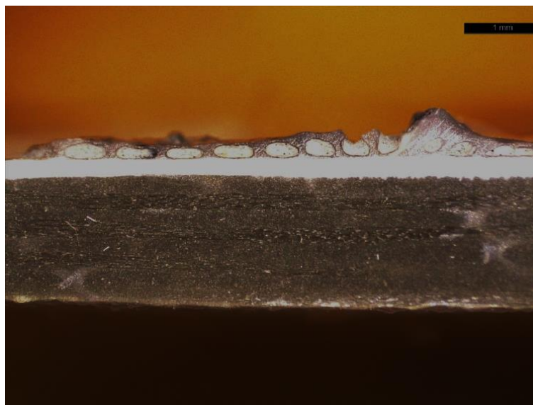
Figure 33: cross section of a sample immersed in the port of Pasaia showing the interface between barnacles and gel coat
