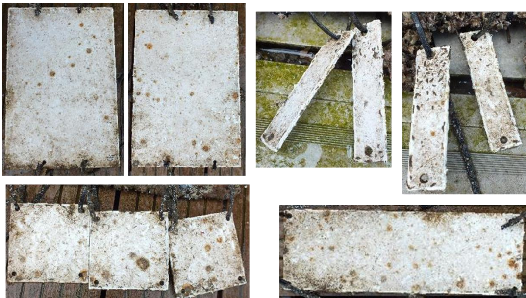
Figure 27: aspect of the samples immersed on the Pasaia port facility after 3 months of ageing
