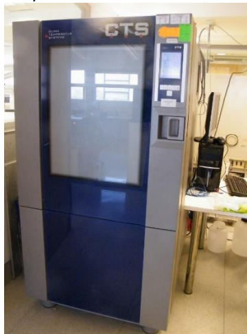
Figure 7: Tecnalia climatic chamber used for the thermal shock ( -2^{\circ}\text{C} )
