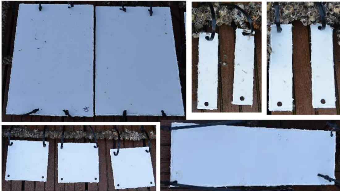
Figure 26: samples fixed on the rack before immersion, Pasaia port, February 2020
